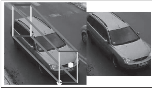
Fig. 4. Ford Mondeo IV Kombi. On the left: calculated bounding box [own study]
