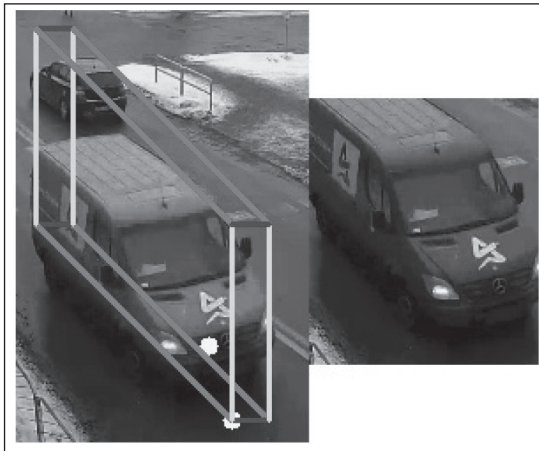
Fig. 5. Mercedes Sprinter 2006. On the left: calculated bounding box [own study]
