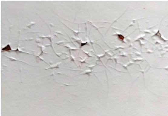
Figure 1. Observed surface treatment defects in FBs. a) orange peel, b) bordered patch (crater), c) wrinkled surface, d) cracking and peeling of the solid coating
