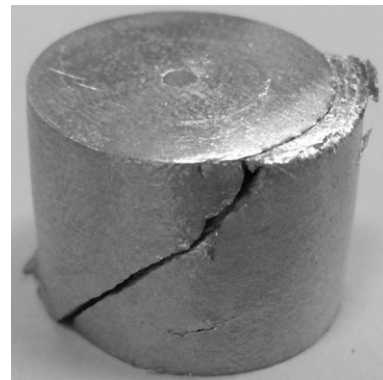
Fig. 5. AZ91 alloy sample after the compression test
