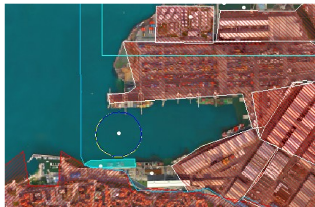
Fig. 5. a) Thermal zones of 12 \text{ kW/m}^2 for ignition of 12 t of gasoline in a pool (Port of Koper)
