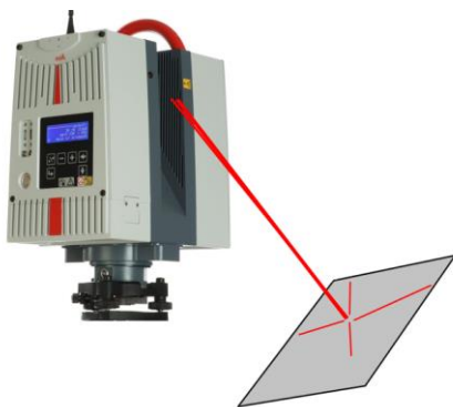
Fig. 4. Principle of operation of a laser scanner and a LIDAR
