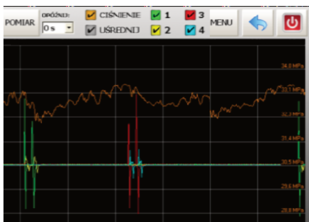
Fig. 6. Current characteristics of injector coils and pressure in the fuel rail.
