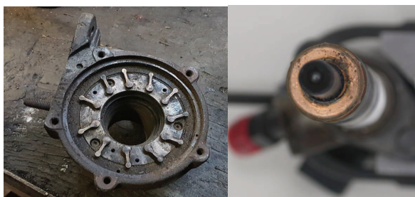
Fig. 7. Residual sediments in the area of the levers positioning the exhaust nozzle blades and in the zone of injector outer openings
