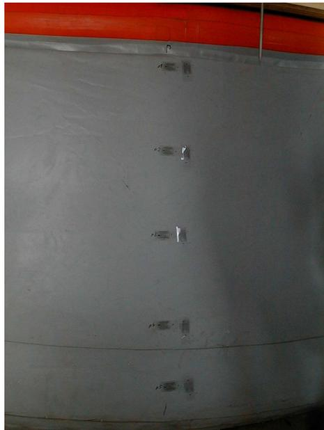
*Fig. 8. Grid sensors glued to FST wall*
