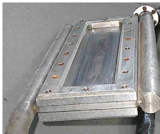
Fig. 2. General view on water cooled EB/X-rays converter with tantalum target design for scanned electron beam (tantalum foil thickness 0.5 mm).
