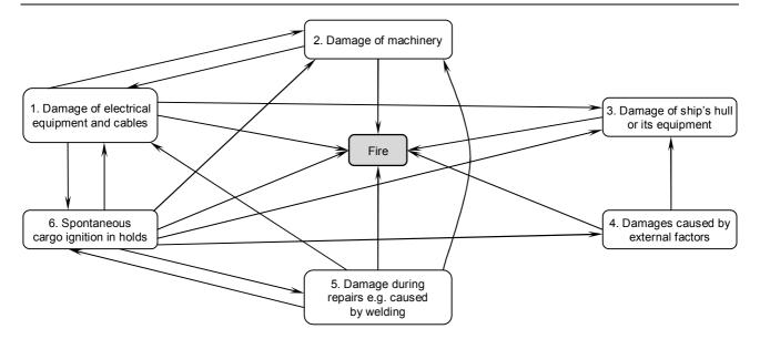
Figure 6. Diagram of interrelationship presenting cause-and-effect links leading to fires on ships
