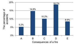
Figure 4. Consequences of fires at sea (A – total damage of a ship, B – a ship rendered unfit to proceed, C – a ship remains fit to proceed, D – fatal accidents or missing persons, E – wounded persons (author's findings based on data for years 2009–2014 (IMO-GISIS, 2015))
