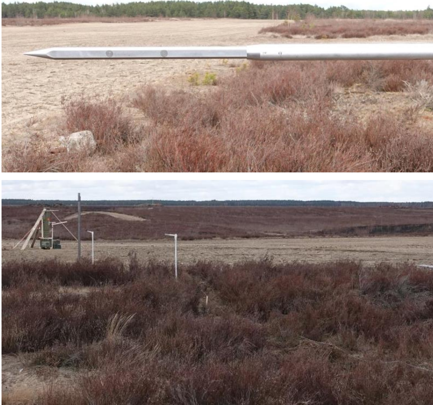
Fig. 16. Top: PCB 137A23 dual pressure sensor — general view. Bottom: method of arrangement of the pressure sensors relative to the warhead. The pipe protection for the sensors can be seen on the left
