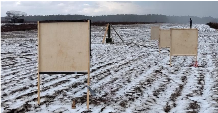
Fig. 9. Layout of flat short-circuit sensors in the field
