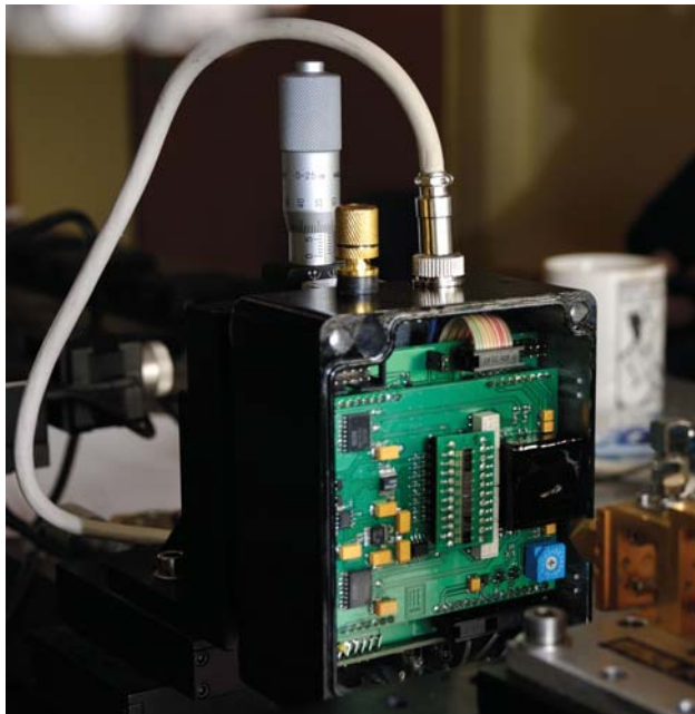
Fig. 15. The hardware part of the second measurement system. The top cover removed for better visibility of internal components. The installed pixel-line (small form factor PCB) can be seen in the center of the upper PCB.
