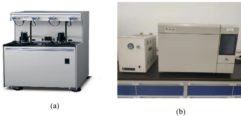
Fig. 2. (a) Autopore IV9500 mercury porosimeter; (b) KSS-5690A series gas chromatograph.
