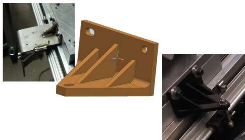
Fig. 3. Design of the element supporting the encoder's sensor
