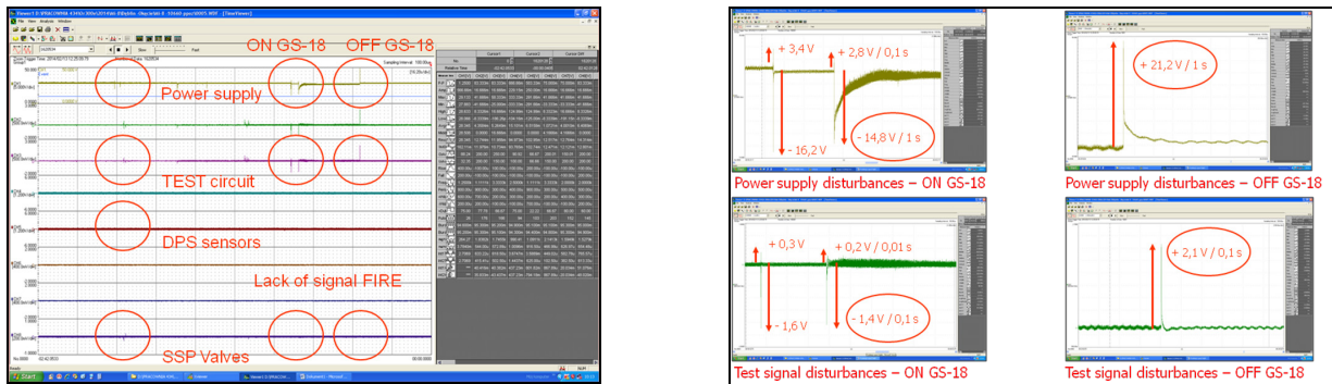
Fig. 2. Electrical interference occurring in the SSP-FK fire suppression system circuits
