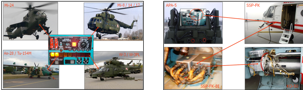
Fig. 1. Aircraft equipped with the SSP-FK fire suppression system
