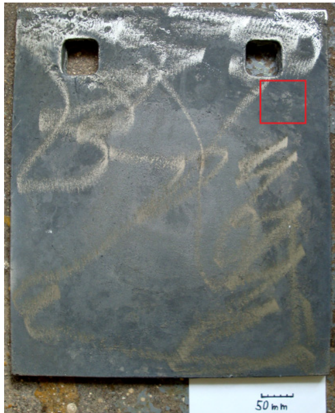
Fig. 1. Experimental casting – protection plate of shot blaster, with marked place of removal of specimens for further examination
