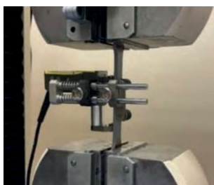
Fig. 4. Sample with extensometer attached
