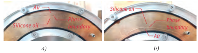
Fig. 6. Position of silicone oil and air inside the damper: a) before starting work, b) after the oil is pushed out by the centrifugal force and the pressure of the inertia ring during operation.
