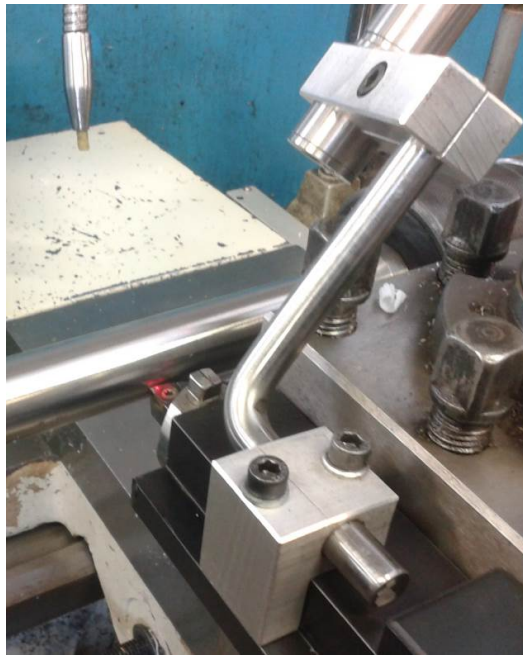
Fig. 1. The laboratory stand for longitudinal turning of external cylindrical surfaces
