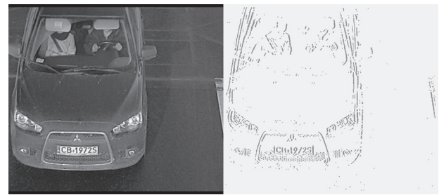
Fig. 6. Input (left) and output (right) of feature extraction method for the plate detector
