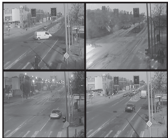
Fig. 3. Examples of incorrect traffic light state classification (CIELAB colour space): top-left: classified as green, top-right: classified as yellow, bottom-left: classified as red-yellow, bottom-right: classified as green
