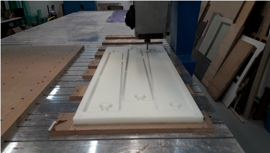
Figure 1. PMI foam during machining to helicopter blade core shape [Zięba M., 2016]
