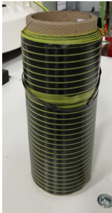
Figure 7. Bobbin of unidirectional prepreg of PARK E-752LT HTS45 12K [Krauze, 2018]
