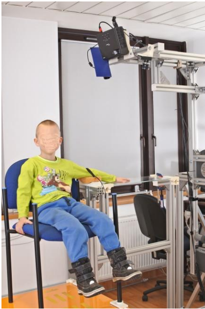
Figure 1. 3D scanner with devices for measuring limbs.
