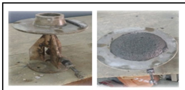
Fig. 2. Flow test of the AAUC mortar
