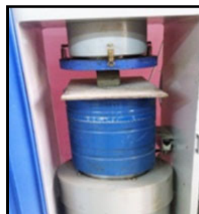
Fig. 3. Compressive strength test of AAUC
