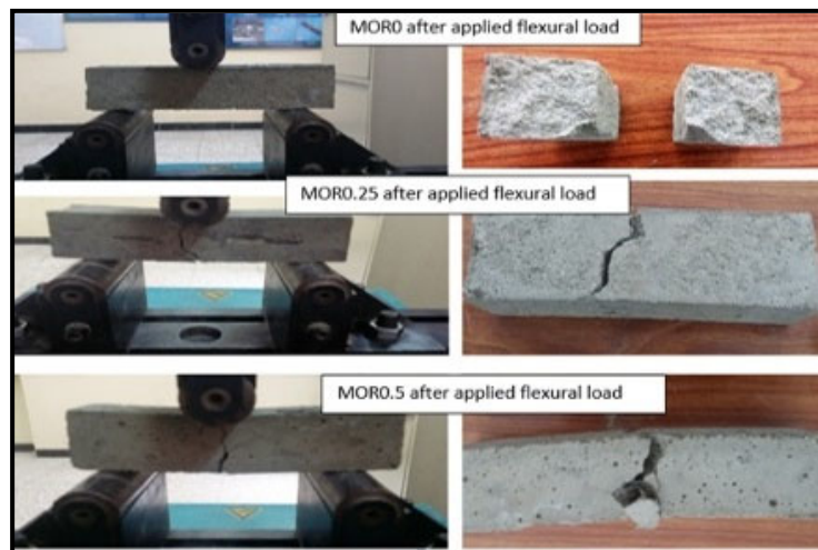
Fig. 17. Mode of failure for AAUC mortar specimens
