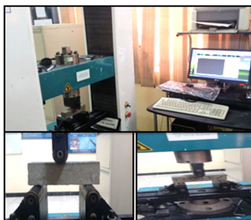
Fig. 4. Flexural test machine
