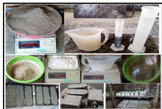
Fig. 1. Production of AAUC mortar
