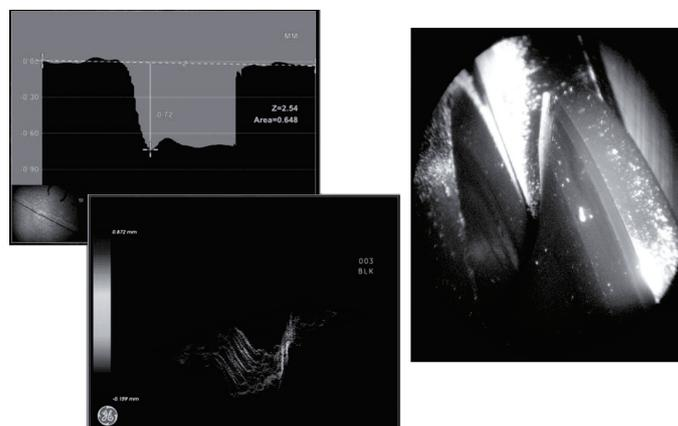
Fig. 5. Defects identified during the measurement phase 3D using industrial videoendoscope XL G3 [3]
