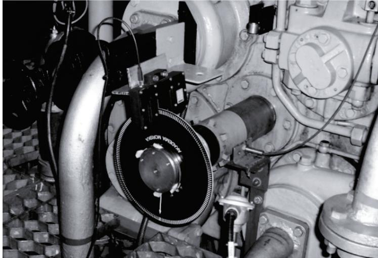
Fig. 2. An optical encoder disc mounted on the engine crankshaft [4]
