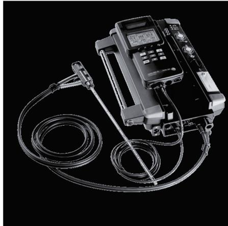
Fig. 6. Portable exhaust gas analyser Testo 350XL [3]
