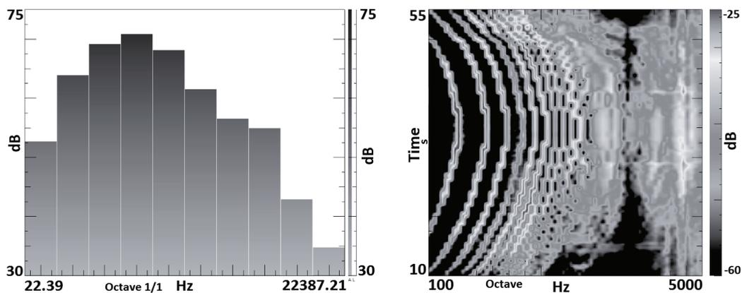
Fig. 3. Examples of measured vibroacoustic signals multiband analyses 1/n octave [11]
