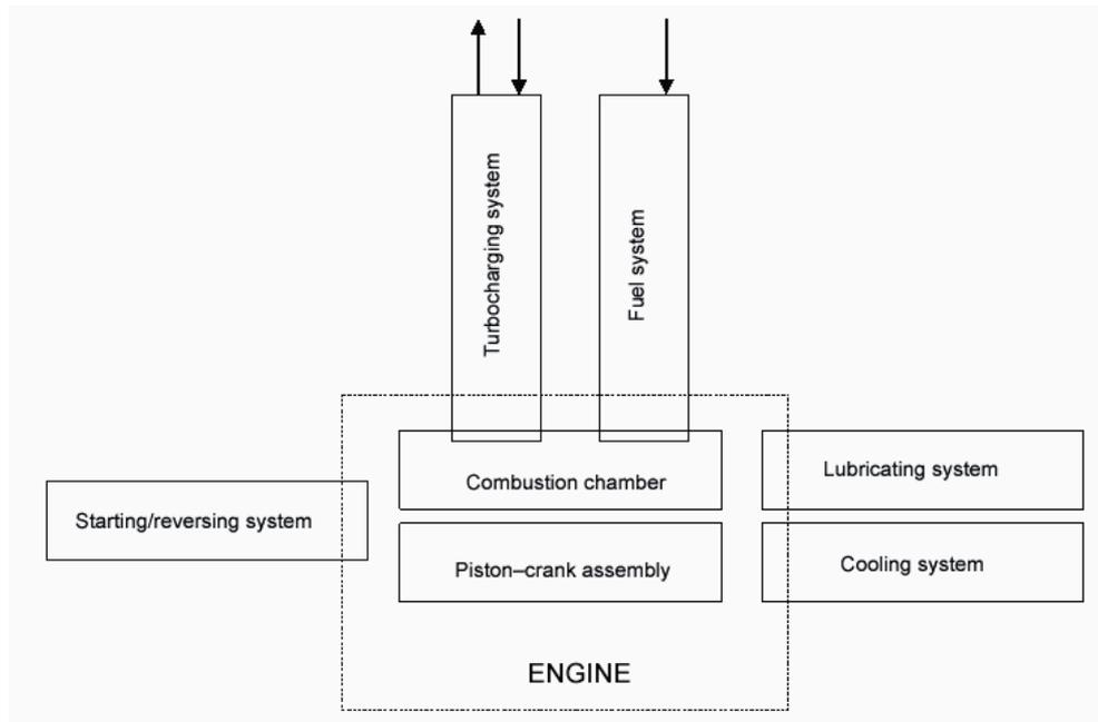
Fig. 1. Fundamental marine engine functional systems [3]
