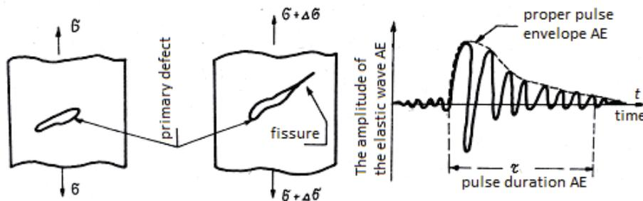
Fig. 4. An illustrative representation of the sample fissure and the related acoustic emission – AE [1]
