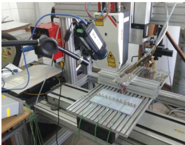
Fig. 2. View of the experimental stand (on the left) and thermocouple placement on samples and 3 types of thermocouple welding to circular channel (on the right)
