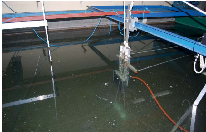
Fig. 6. Parametric echosounder antenna on support
