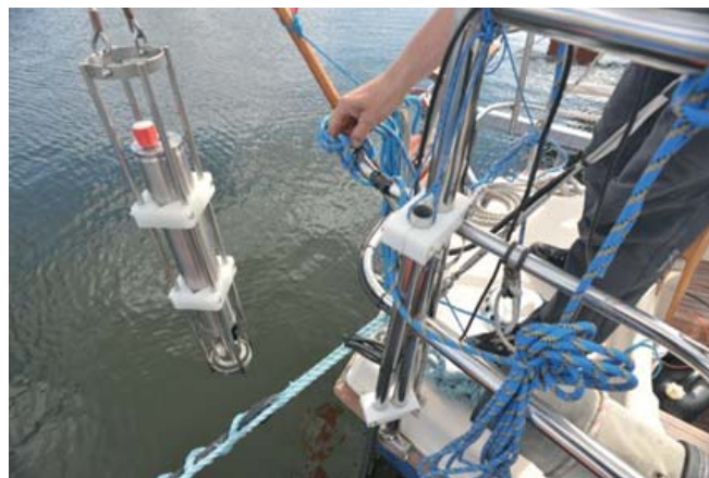
Fig. 2. Sound velocity probe - MIDAS
