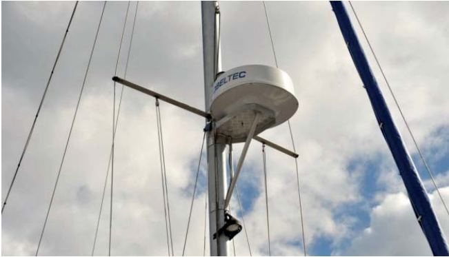
Fig. 4. Navigation device – radar
