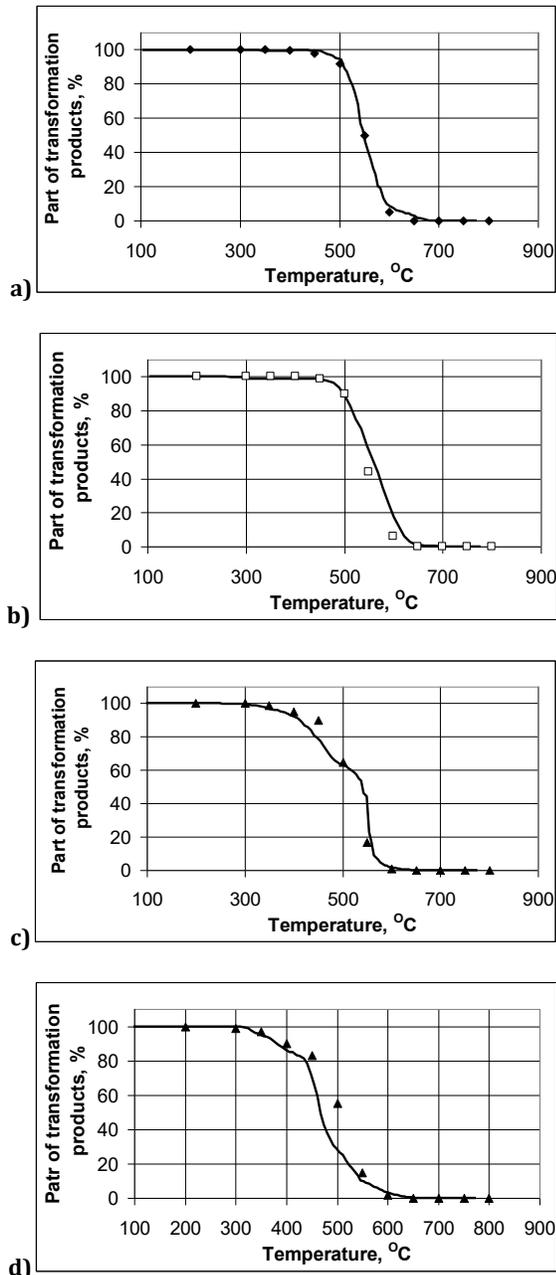
**Fig. 1 Comparison of calculated kinetic curves (given as solid lines) of austenite transformation with experimental data (given as points) at different constant cooling rates: a) 5 °C/s, b) 10 °C/s, c) 17 °C/s, d) 30 °C/s**
