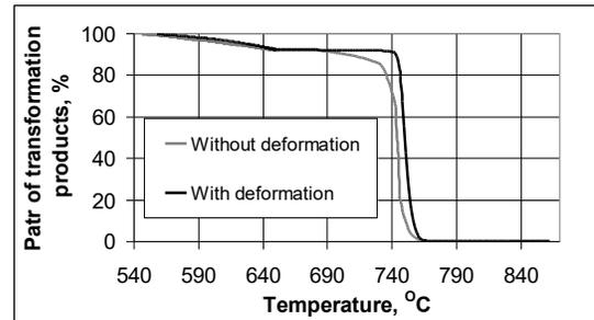
**Fig. 2 Simulated cooling curves of austenite transformation during studied cooling regime**
