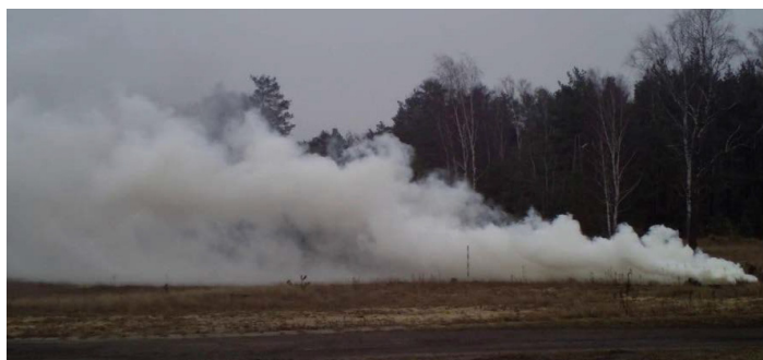
Fig. 3.6. Smokescreen in visible light — first smokescreen section with a length of up to 25 m. Test object invisible. Screen height of about 3 m at a distance of 10 m from the smoke source [9]
