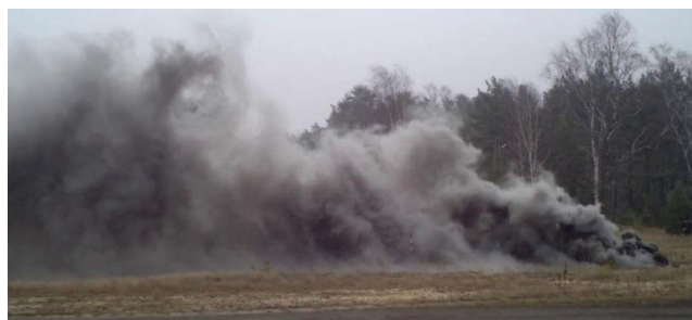
Fig. 3.9. Smokescreen in visible light — first smokescreen section with a length of up to 25 m. Test object invisible. Screen height of about 5 m at a distance of 10 m from the smoke source [9]
