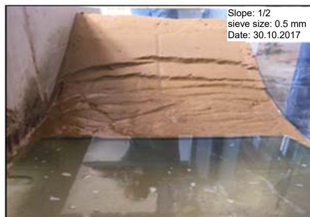
Fig. 14. Failure of the experimental model dam, crest width – B = 5 cm; source: own study
