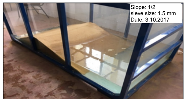
Fig. 6. Seepage water of the experimental model dam; source: own study
