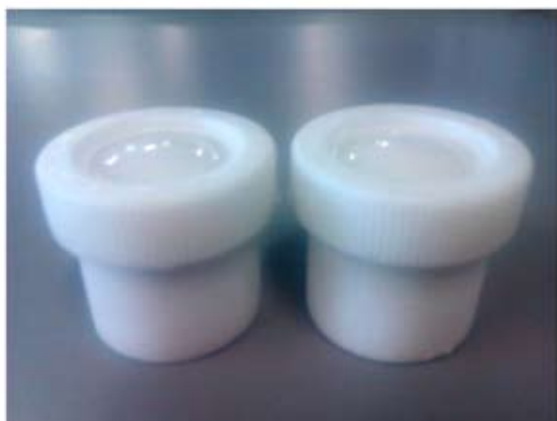
Fig. 1. Cuvettes used for determination of release rate of active ingredients from cosmetic formulations
