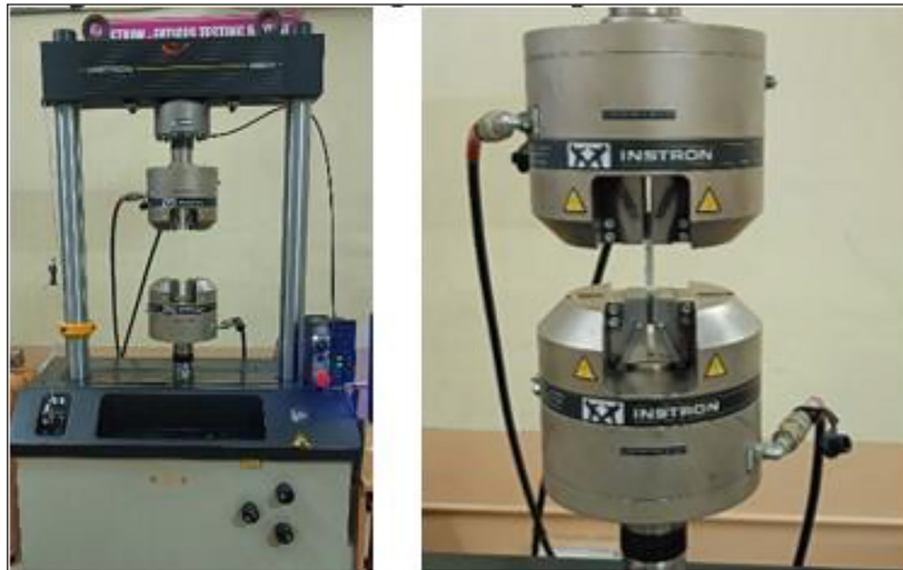
Figure 12. Tensile test set up
