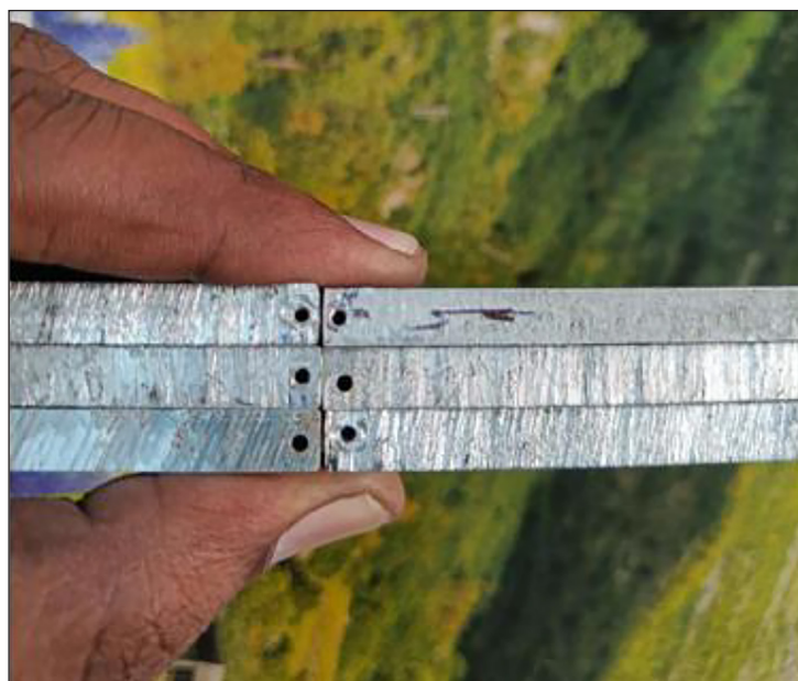
Figure 4. Samples with holes along stir zone for powder addition
