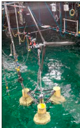
a) Scaled model of OC4-DeepCwind platform in MARIN (Hall & Goupee, 2015)
