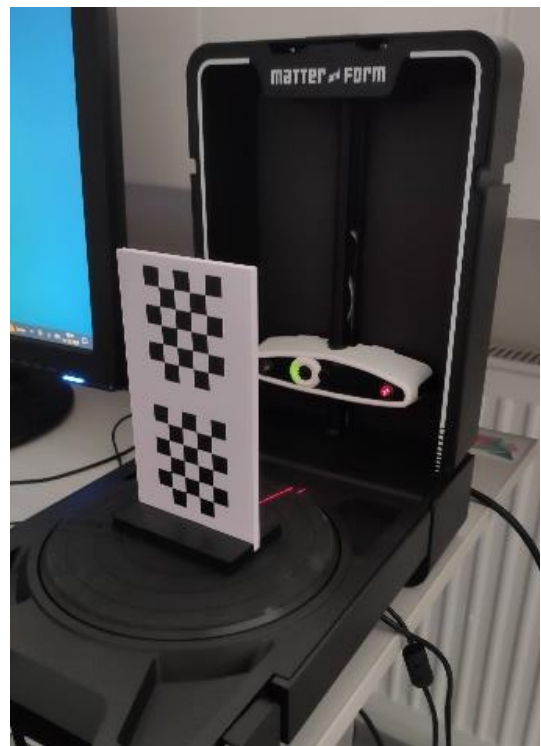
Fig. 2. Used 3D scanner and its calibration process (authors).
