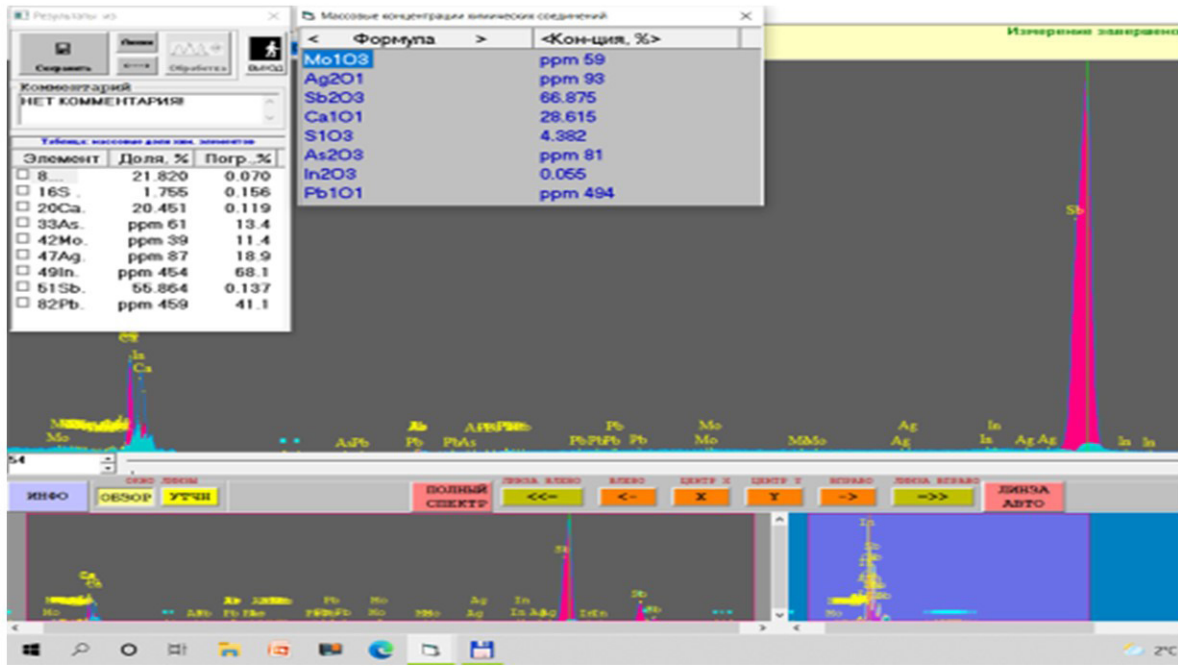
Fig. 7. X-ray fluorescence diagram of flame-retardant sample 3
