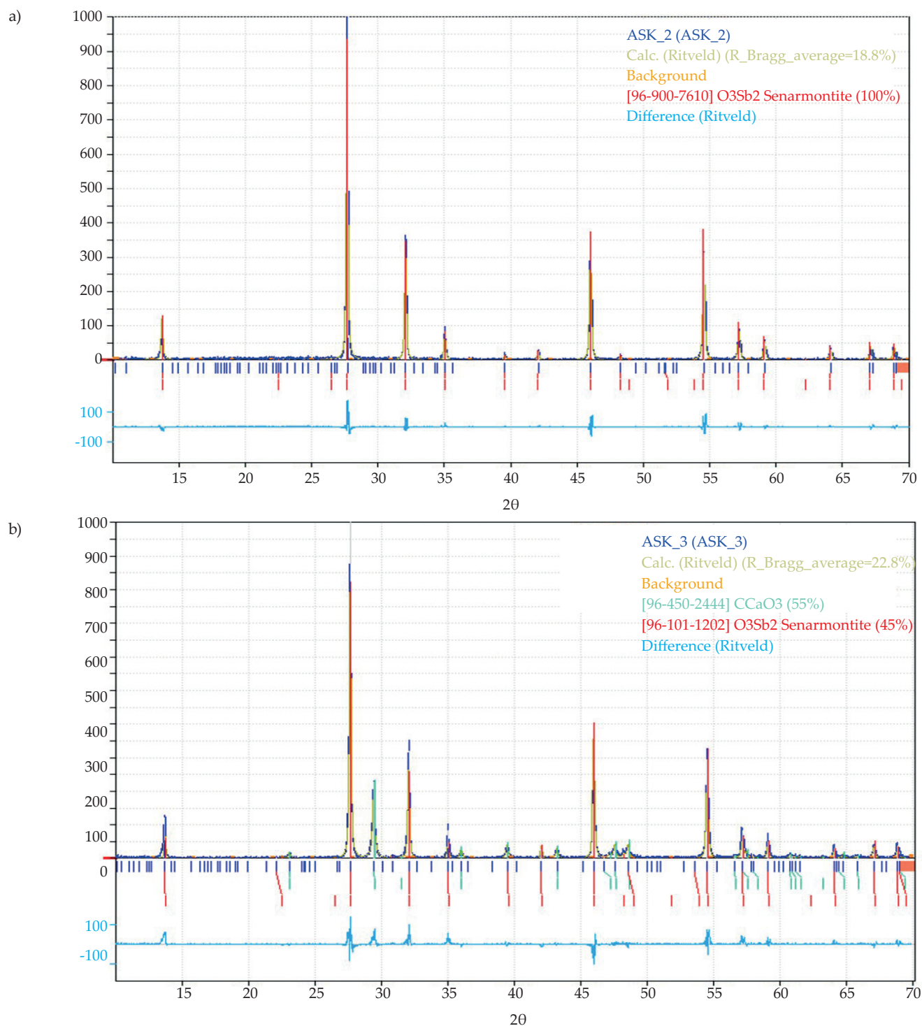
Fig. 6. Diffraction patterns of flame retardants: a) sample 2, b) sample 3
