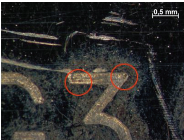
Fig. 8. Examples of pitting at the site of the implant marking
