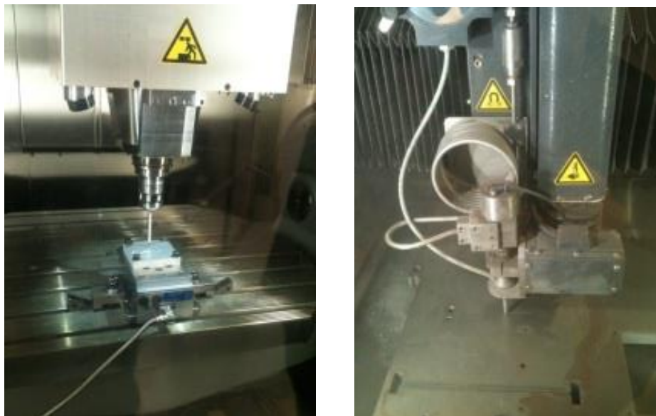
Fig. 1. Milling setup (left) and waterjet head (right) used during experiment
