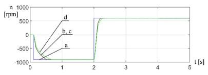
Fig. 7. Response of a control system with introduced additive disturbing signals for 1kHz on the level b = 10%; c = 50%; d = 100% for the set step of rotational speed and load step in the 4<sup>th</sup> second of simulation – a
