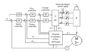
Fig. 1. Direct field-oriented control system (DFOC) [3, 4, 5, 7, 8, 10]
