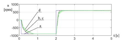
Fig. 6. Response of a control system with introduced additive disturbing signals for 1Hz on the level b - 10%; c - 50%; d - 100% for the set step of rotational speed and load step in the 4<sup>th</sup> second of simulation – a
