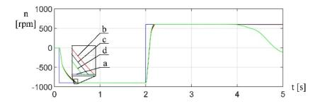
Fig. 5. Response of a control system with introduced additive disturbing signals for 1Hz on the level b - 10%; c - 50%; d - 100% for the set step of rotational speed and load step in the 4<sup>th</sup> second of simulation – a
