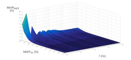
Fig. 4. Dependency of the parameters of an additive sine-wave disturbing signal (frequency f and the contents of this disturbing signal in the basic signal MAPE<sub>IN</sub>) on the level of disturbances in the output signal MAPE<sub>OUT</sub>
