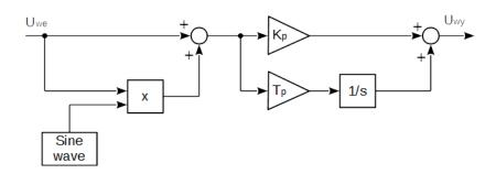
Fig. 3. Diagram of the controller with sine-wave disturbances in the input signal:  $U_{we}$  – input signal of the controller;  $U_{wy}$  – output signal of the controller:  $K_p$  – controller boosting;  $T_p$  – coefficient dependent on integral action times
