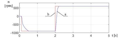
Fig. 2. Waveforms of rotational speed: the set process (b) and the process executed by the control system based on the calculated parameters of PI controllers (a)
