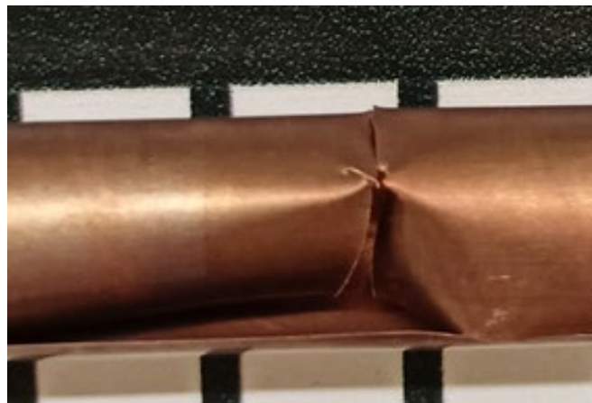
Figure 11. Plastic deformation results received in a laboratory test (photo: T. Pałgan)
