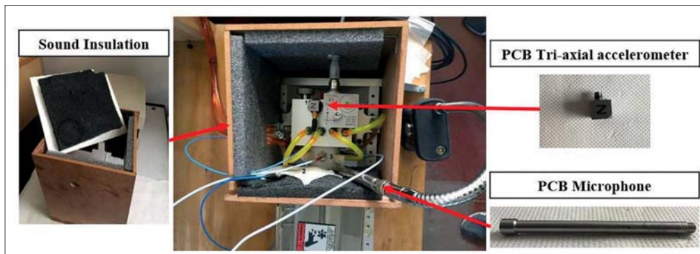
Fig. 3. Sensor installation and experimental setup
