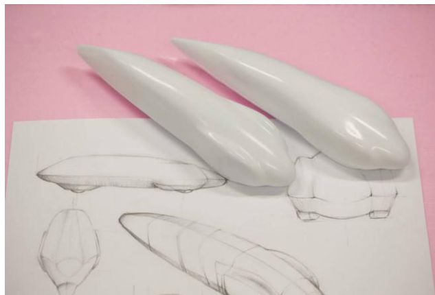
Fig. 1. 3D printed, conceptual models of hydros [source: own study]
