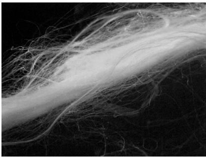
Figure 3. Luminescence of prepared cellulose fibres under ultraviolet irradiation ( \lambda_{ex} = 254 \text{ nm} ).
