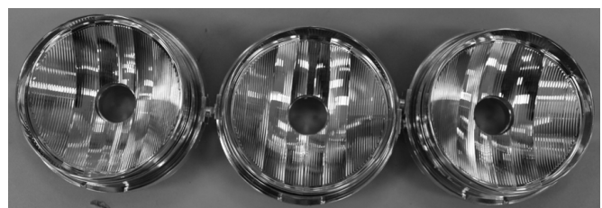
Fig. 6 After 120 hours no visible damage has occurred on tested samples
