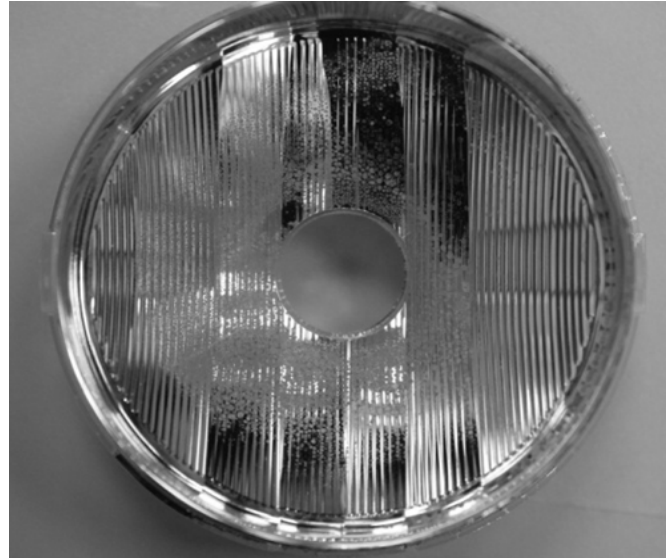
Fig. 5 Visible damage of reflective aluminium layer
