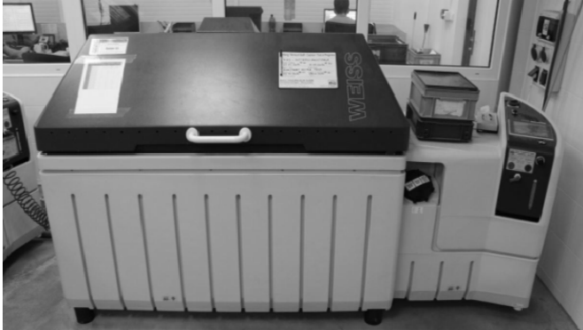
Fig. 2 Testing device – constant climate chamber
