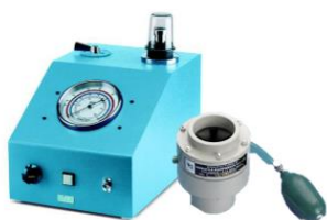
Fig. 3. DISA type permeability testing machine and accessory for measuring cores
