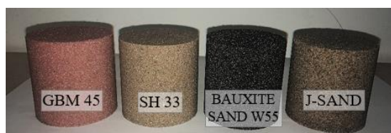
Fig. 4. Standard permeability test specimens
