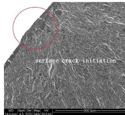
(b) Single crack initiation ( N_f = 7.12 \times 10^6 )
