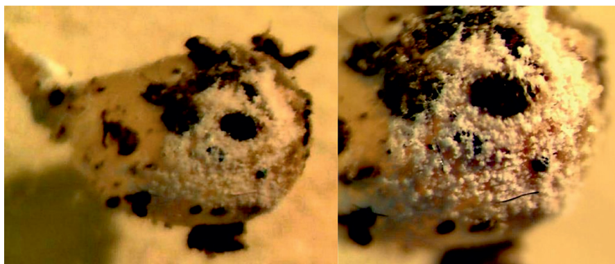
Fig. 8. Covering of the M_b -1 cellulose granule with salt (photos taken by hand).
