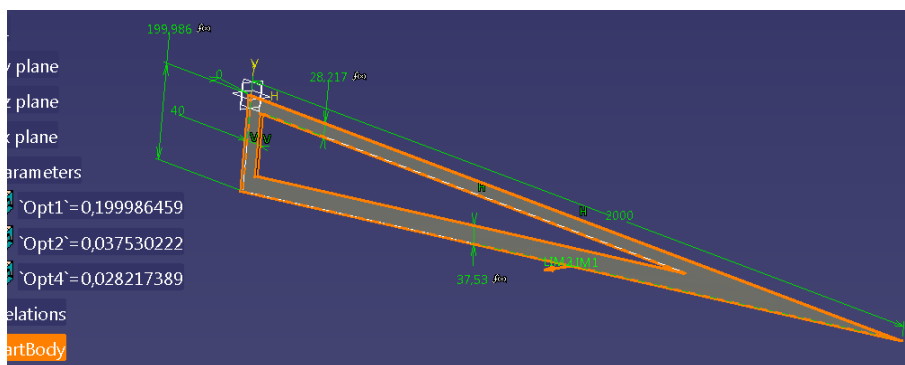
Fig. 14. Triangular I Profile Cantilever Beam with a Triangular Hole [source: own study]
