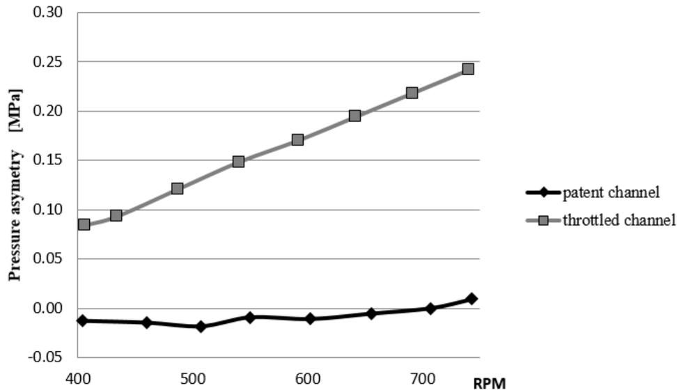
Fig. 5. Effect of channel throttling on compression curve asymmetry
