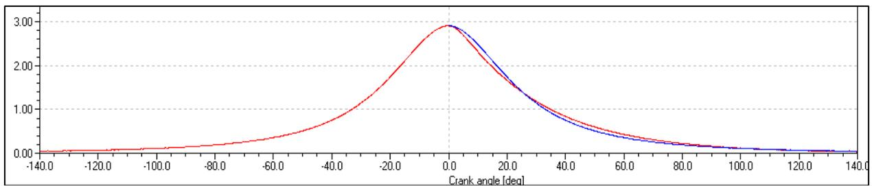
Fig. 2. Comparison of the expansion curve with the mirror image of compression curve
