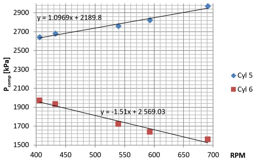
Fig. 1. Cylinder compression pressure as a function of engine speed for patent channel (cyl. 5) and channel choked by plate with orifice (cyl. 6)
