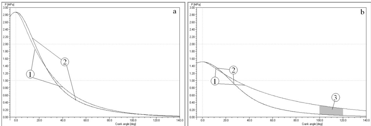
Fig. 4. The measurement of the asymmetry of compression curve with no load at engine speed 700 RPM: a) for the clean channel b) for channel partly choked: 1) the expansion curve, 2) the mirror image of the compression curve 3) measure of the asymmetry
