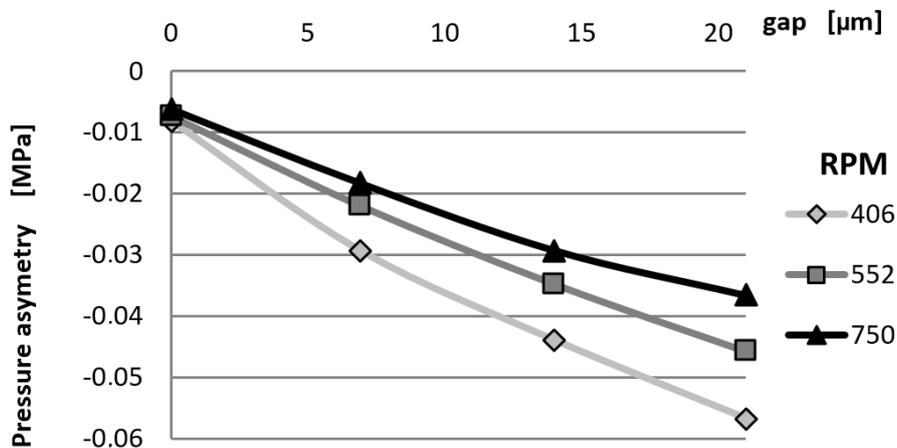
Fig. 3. Effect of gasses leaks and engine speed on compression curve asymmetry
