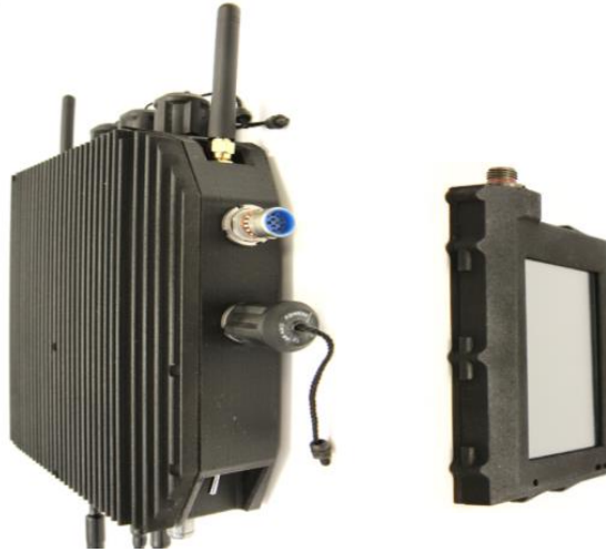
Fig. 1. A photograph of the Modular Integrator for soldier's C4I system management, including a display
