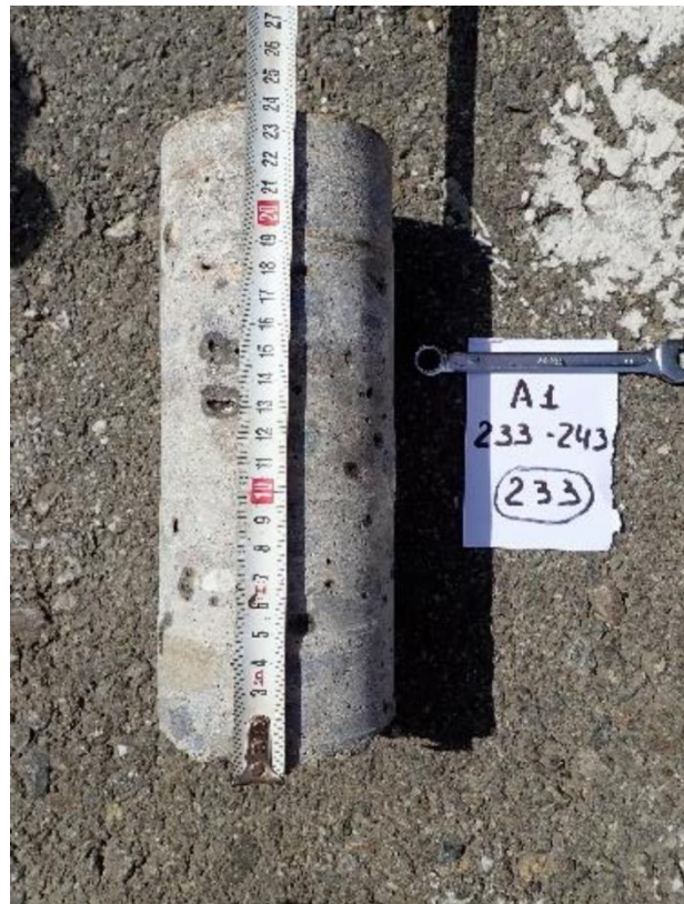
Fig. 2. An example of cores taken on the A-1 «Astana – Petropavlovsk» highway km 233
