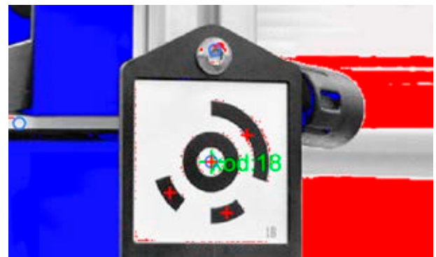
Figure 8. An example of the segments that were prequalified as potential markers (blue circles and red crosses)
