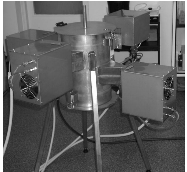
Fig. 2. View of the layout of microwave generator chamber with arrangement of microwave coupling systems
